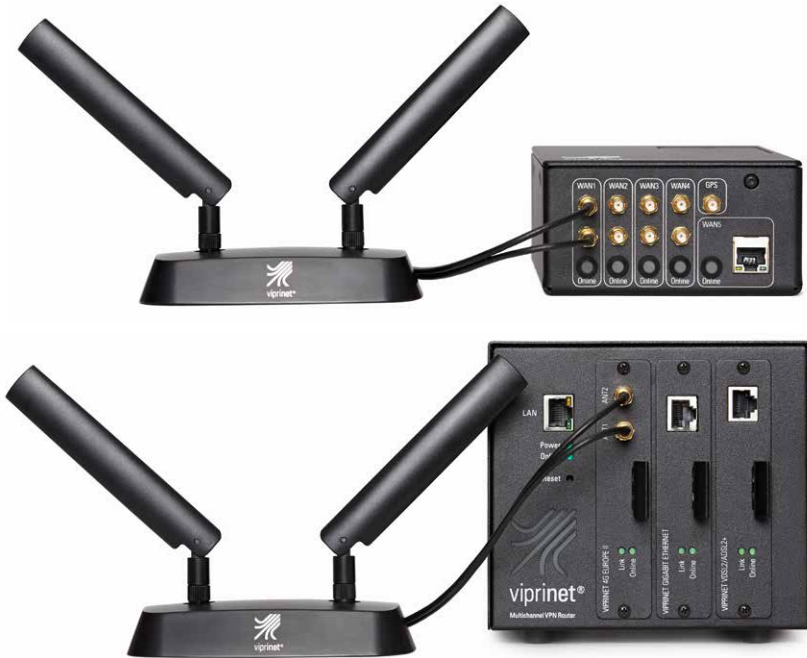
Figure 4.1 Connecting antennas to your router
