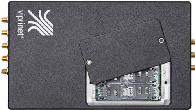
Figure 4.2 Removing the SIM module cover plate
