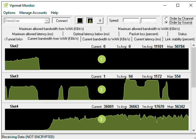
Figure 6.4 A screenshot from the Monitor and the related menu from the AdminDesk showing extra high-cost channels being brought in to satisfy circuit load when an affordable channel becomes unreliable. (Rugged VPN firmware)
