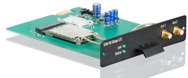
The "4G Global LTE" module provides global mobile connectivity in your Viprinet Multichannel VPN Router. Although the module "only" operates in LTE category 4, and thus has a maximum downstream of 150 Mbps, it supports so many radio bands that it is extremely future-proof for national and international use. All LTE bands currently used in Europe and those planned for the future are covered, as are most of the other frequencies used internationally.
