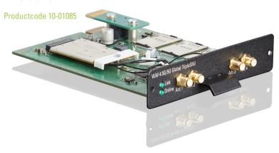
This 5G module is designed for today's and upcoming 5G networks in Europe, the Americas and other regions. The module supports both the mixed-mode combination of LTE+5G networks (also called "5G Non-Standalone") being in deployment today, and also using "pure" 5G (also called "5G Standalone") which is to be rolled out in various countries.
