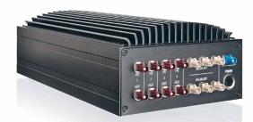
A Gigabit Ethernet interface provides the aggregated bandwidth to the LAN. At the same time, the two integrated WLAN access points with 2.4 or 5 GHz provide the available bandwidth without cables. Using the LAN interface, Toughlink can be supplied with power via PoE+. Therefore, if the device is mounted outside a building or vehicle, it only requires one single (Ethernet) cable to supply the interior.
